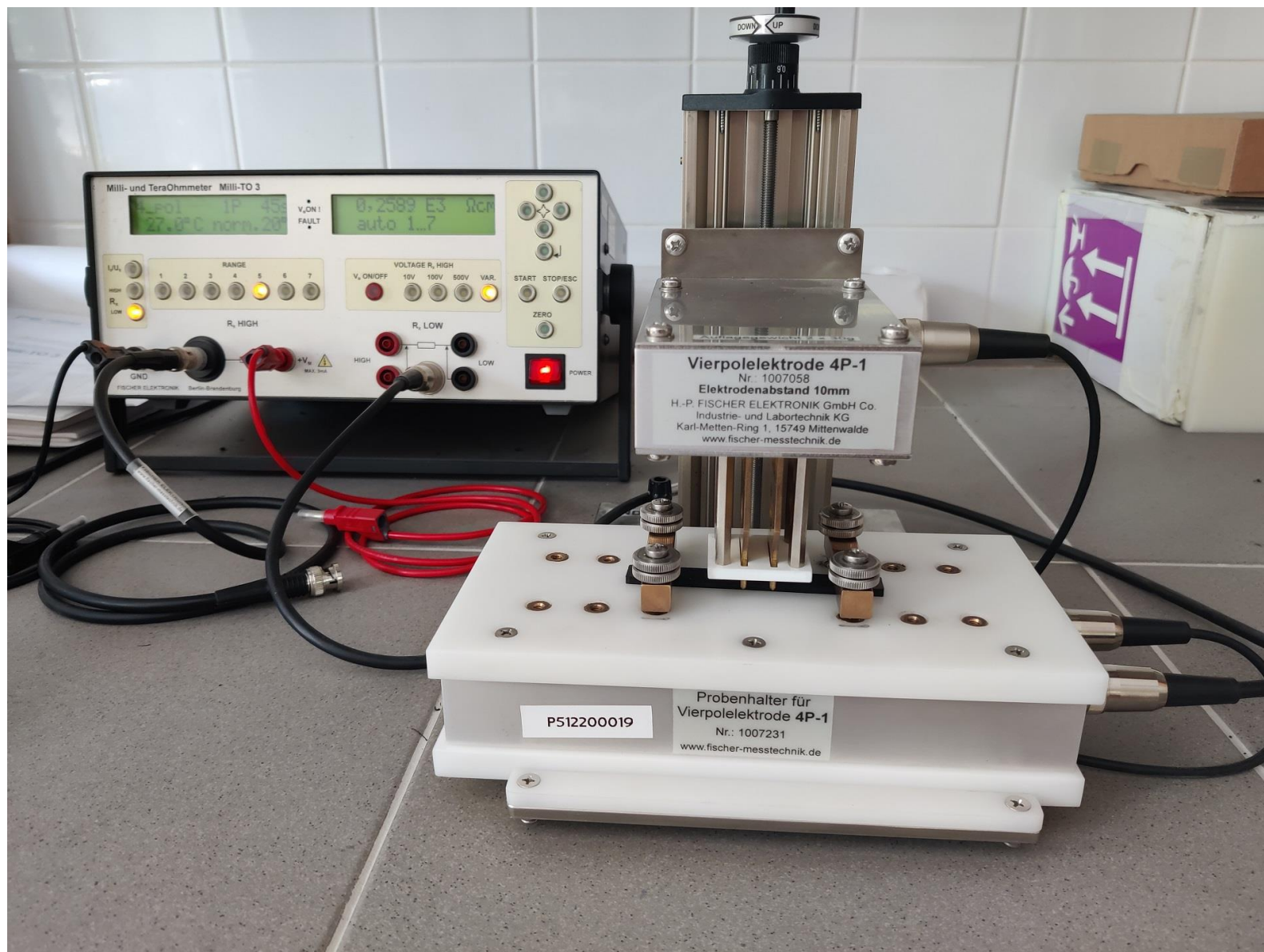
Figure 1: Test illustration - Milli-TO3 ohmmeter connected with four-pole electrode 4P-1
